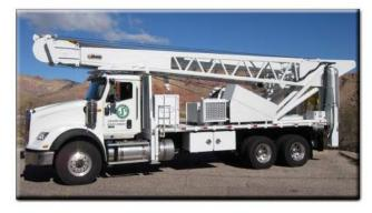
The 60T has a pulling capacity of 120,000 lbs. The hoist is designed for fast and easy setup by means of a self supporting mast with two 6" bore hydraulic cylinders. A guy cable system is not needed in most situations.
