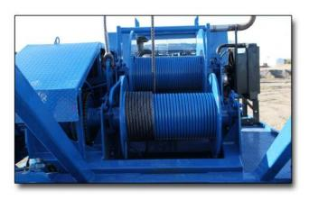
Both the mainline and optional sandline use motors that are hydrostatically driven with infinite variable speed control for exceptionally smooth operation. These motors include an internal braking system.
