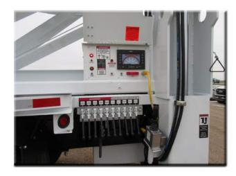
Controls are conveniently located at the left rear corner of the machine in close proximity to the work area.
